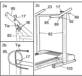
With the help of a second person, carefully tip the Uprights (82) down as shown. Note: It may be helpful to place a foot on one of the Wheels (95) as you tip the treadmill.
